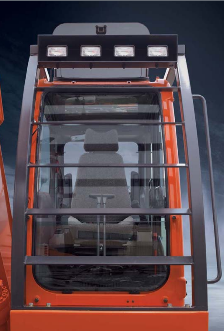
Cabin protector To perfectly protect a driver from a dangerous object such as wood or stone, a guard is equipped at the upper and front part of the cabin.(Meeting international standard ISO 10262) Equipped with 4 lamps at the upper part of the guard, it is convenient to work at night.
