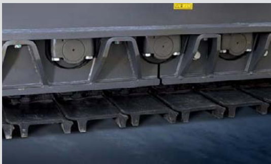
Low roller With improvement of lower roller body internal structure, and strict test verification of reliability, it has secured a higher level endurable quality, and a full guard was applied to protect the lower roller and prevent the derailment from a track at a rugged area work.
