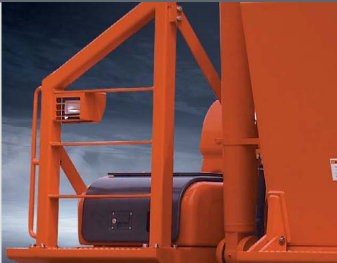
Cabin protector To perfectly protect a driver from a dangerous object such as wood or stone, a guard is equipped at the upper and front part of the cabin.(Meeting international standard ISO 10262) Equipped with 4 lamps at the upper part of the guard, it is convenient to work at night.
