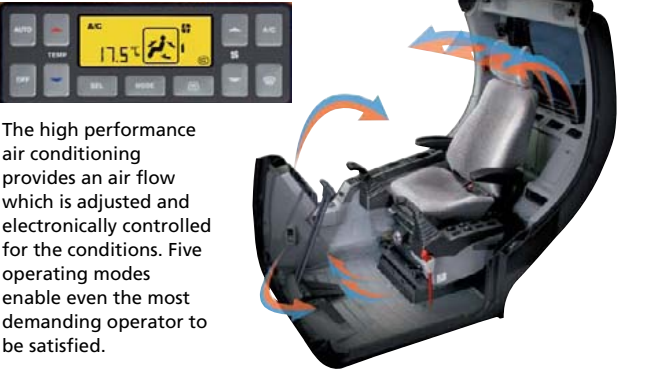
Air suspension seat (opt) Equipped with various functions of adjustment forth and back and, and lumbar support, it reduces the vibration of equipment transmitted during work in an effective way. Also for considering winter working environment, Seat warmer functions equipped.
