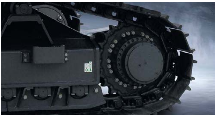
Travel motor Running drive force improved with the efficiency improvement of the running device, its performance is excellent at a slope or swampy area.
